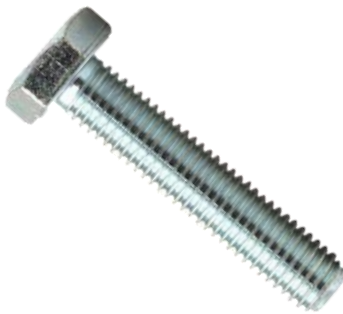
Set Screw Grade 8.8 Zinc Plated DIN 933
