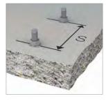
Reduction factors related to the fixing spacing: fs
