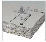
Reduction factor related to the distance  $c_{cr,sp}$  of the fixing from a corner:  $fc_{cr,sp}$
