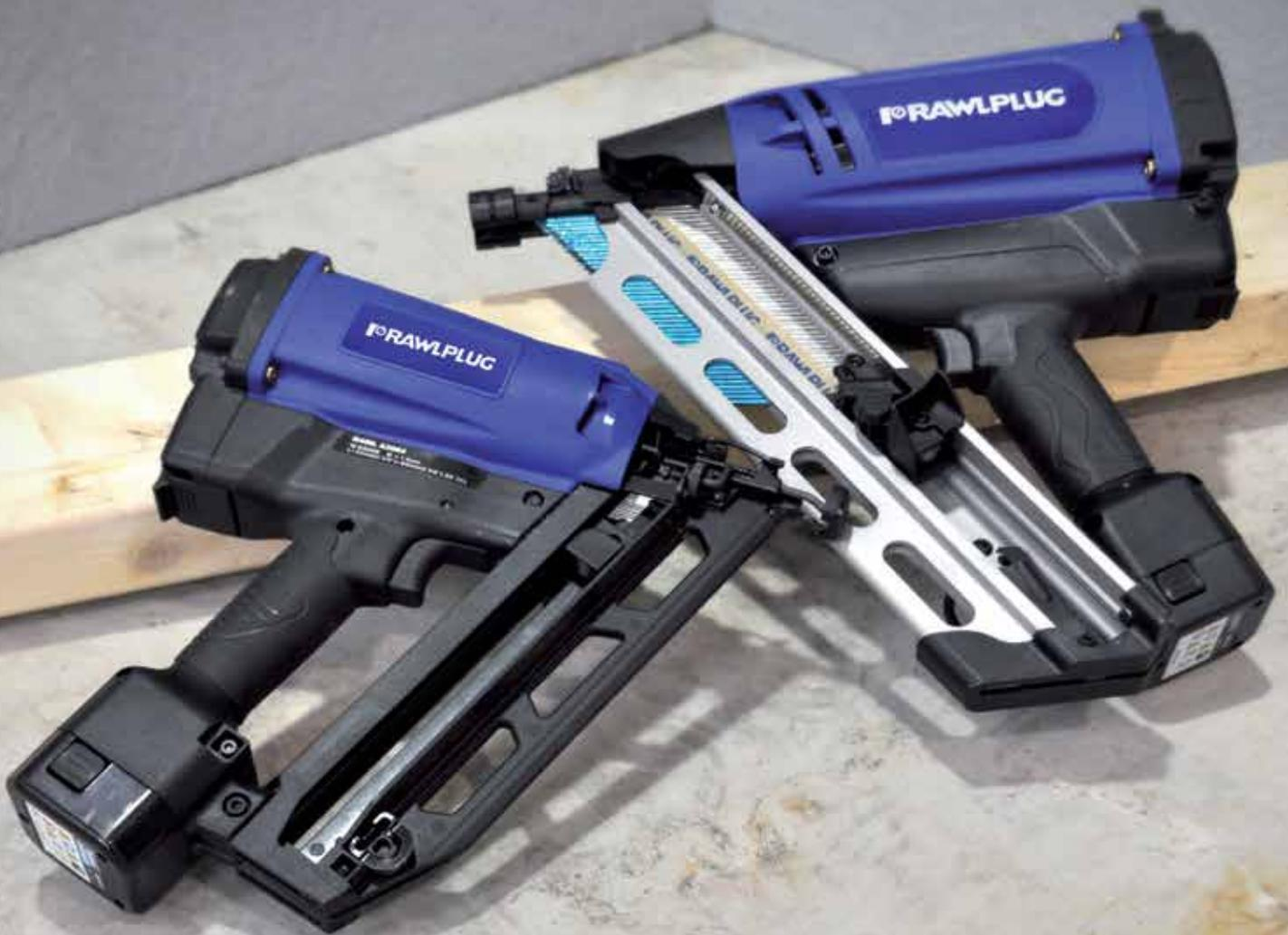
The WW90CH is a gas powered framing nailer for using clipped head nails. The tool will function with plain or ring shank nails ranging from 50 to 90 mm in length. It has a magazine capacity of 60 nails and features a quick loading mechanism and clip to prevent nails from dropping out when reloading.
